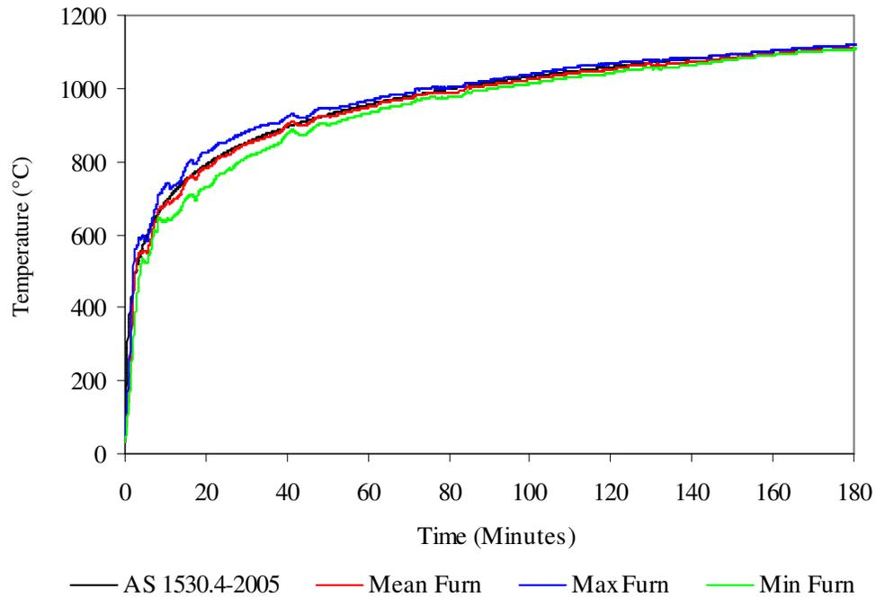
Figure A5.1: Furnace Temperatures vs. Time.
