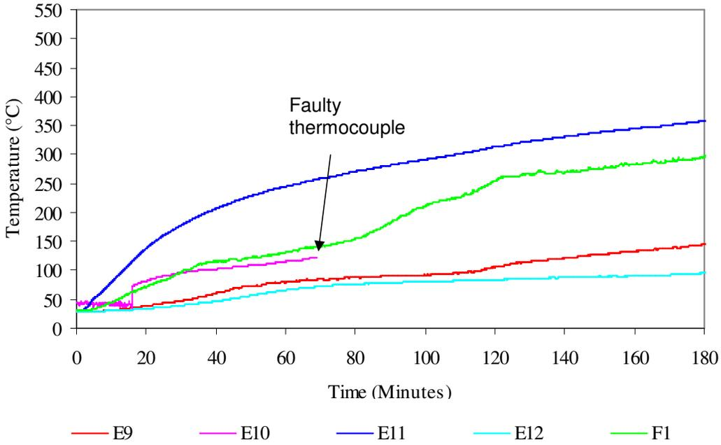
Figure A5.9: Service G. Temperatures vs. Time
