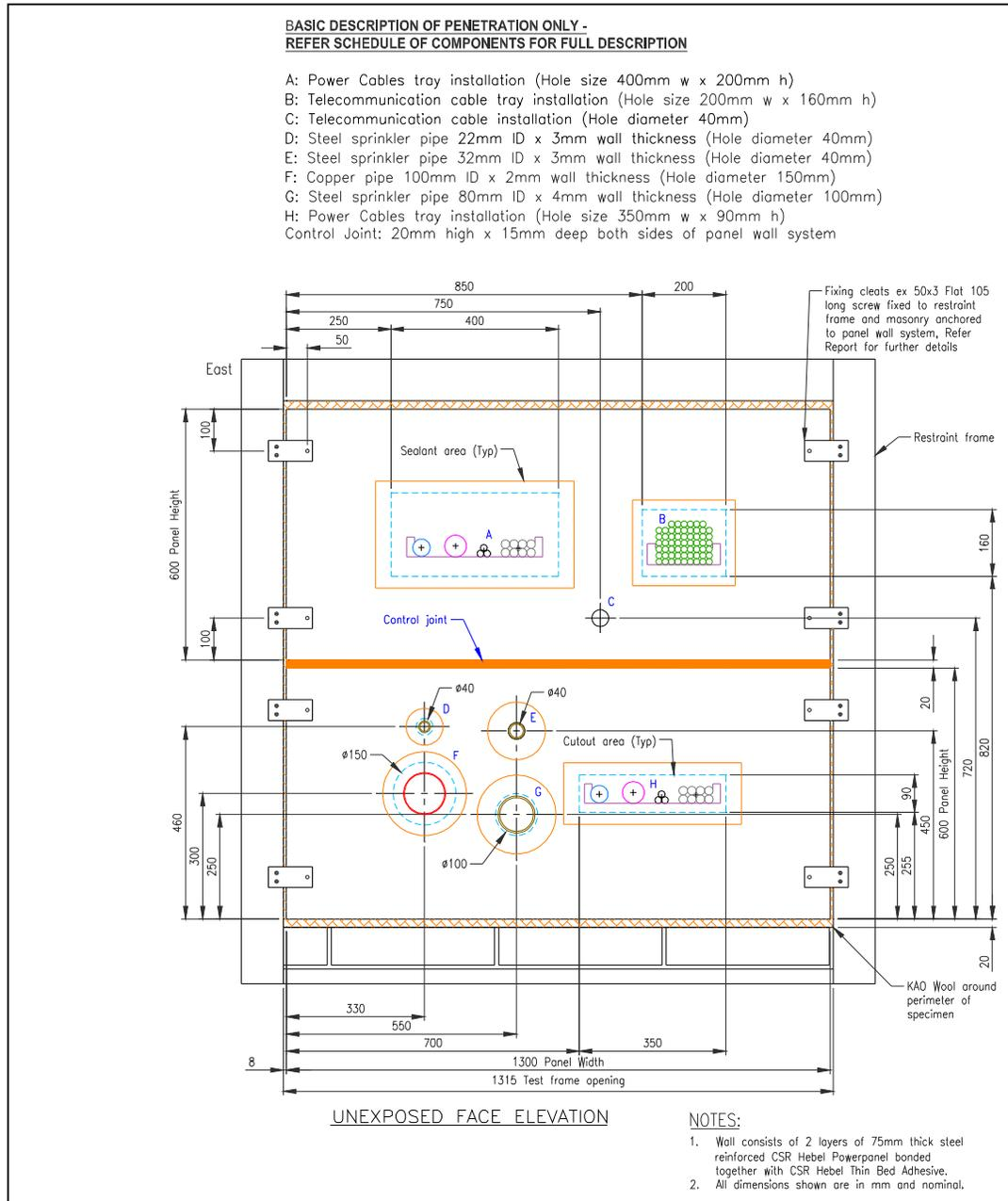
Figure A1.1: Elevation of Test Specimen
