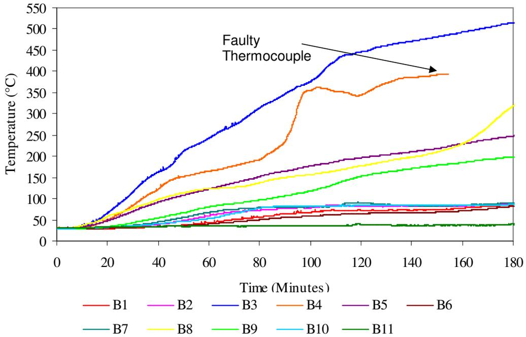
Figure A5.2: Service A. Temperatures vs. Time
