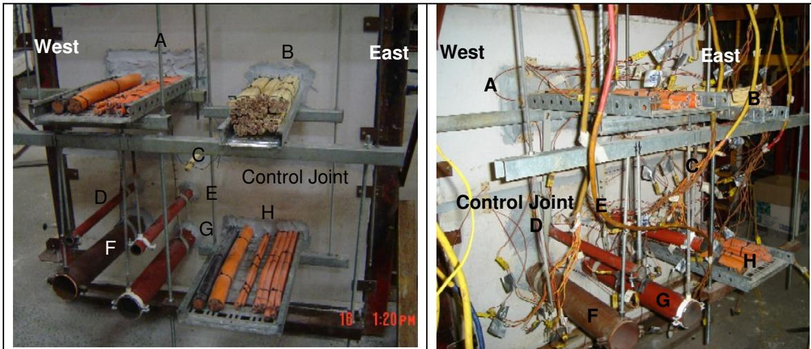
Figure A6.2: Unexposed face of test specimen prior to commencement of the test.
