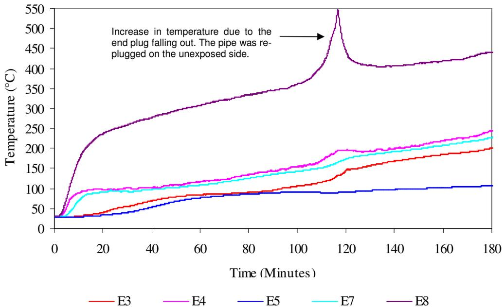
Figure A5.7: Service F. Temperatures vs. Time
