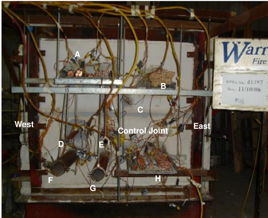
Figure A6.3: Unexposed face of test specimen prior to commencement of the test.
