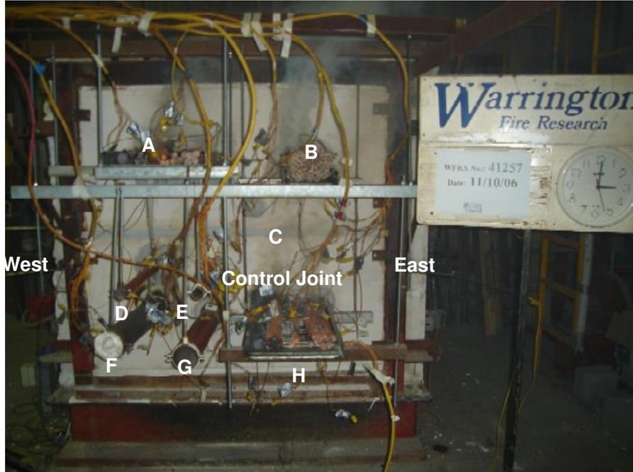
Figure A6.5: Unexposed face of test specimen after the completion of the test.
