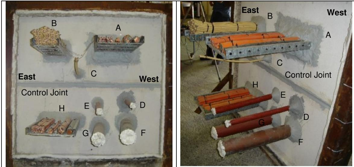
Figure A6.1. Exposed face of test specimen prior to commencement of the test.
