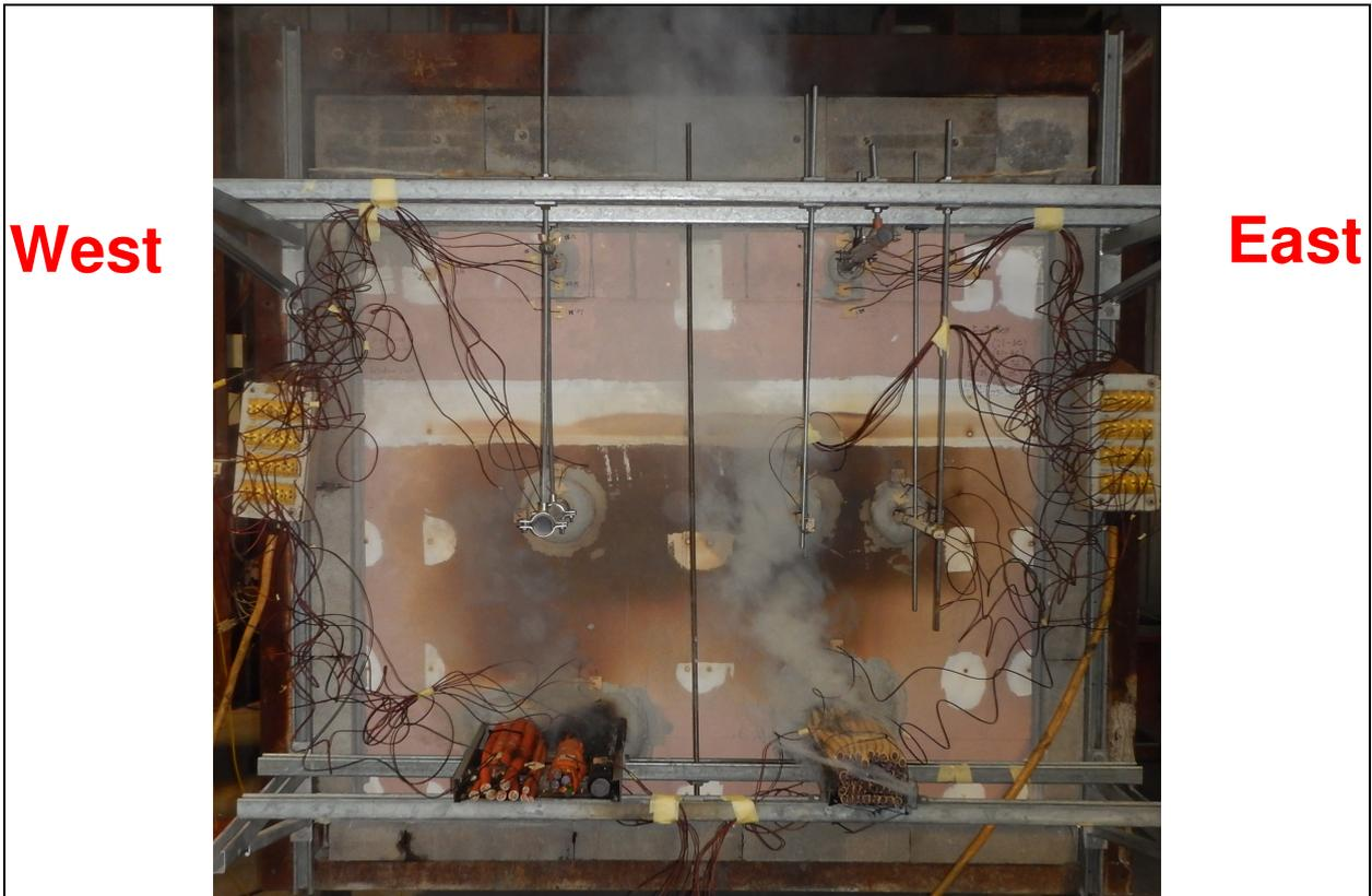
Figure A6.3. Unexposed face of specimen at the end of the fire-resistance test.
