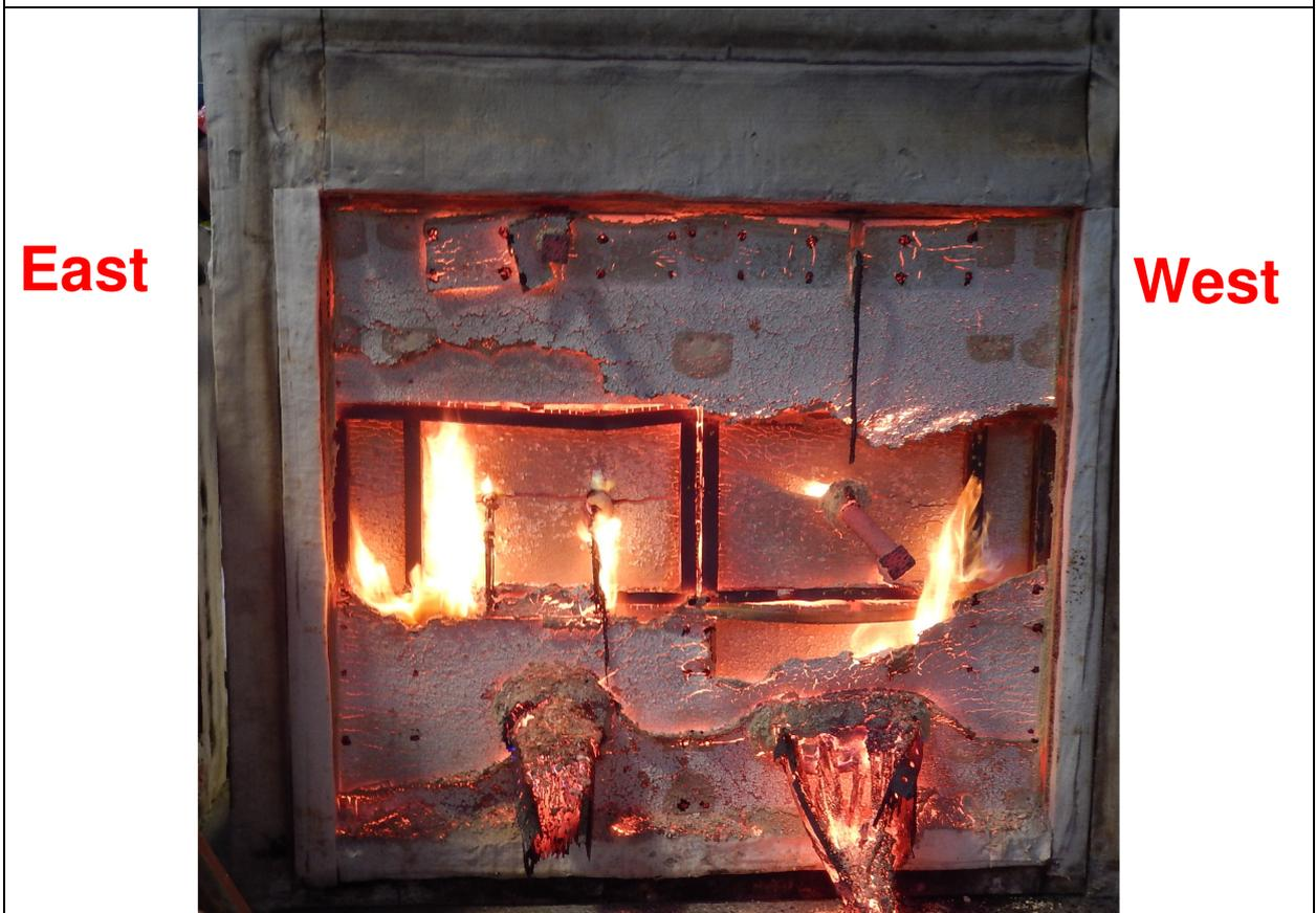
Figure A6.4. Exposed face of specimen after the end of the fire-resistance test.
