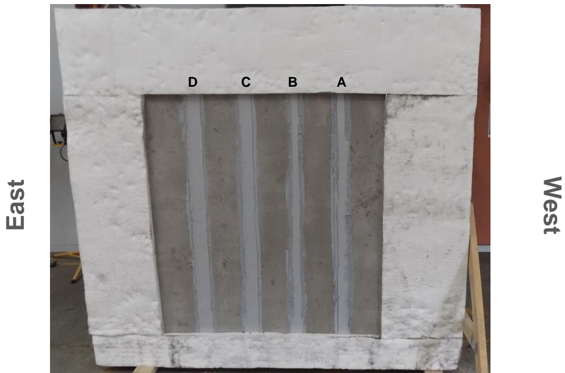
Figure 14 Exposed face of the specimen before the start of the test
