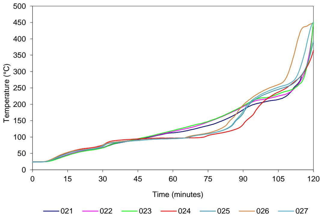
Figure 9 Penetration system B – temperature vs time
