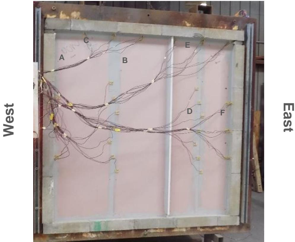
Figure 14 Unexposed face of the specimen before the start of the test
