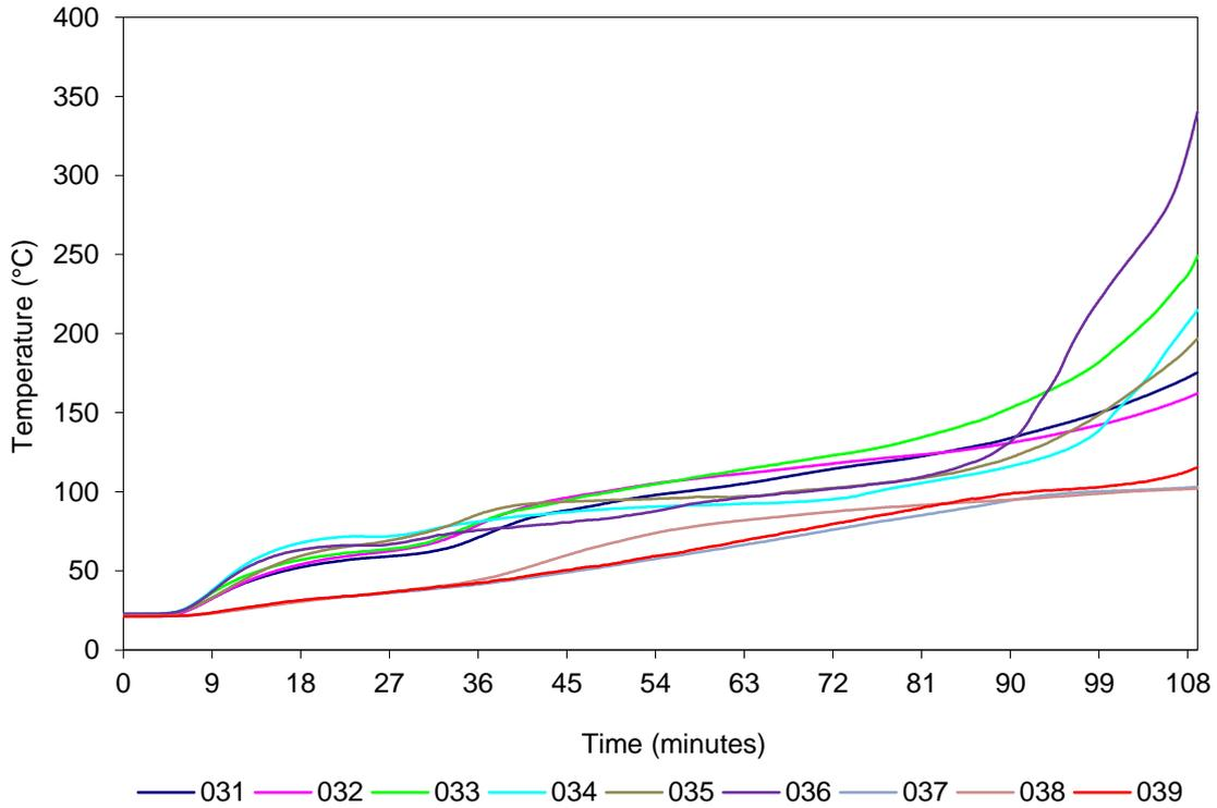
Figure 10 Penetration system C – temperature vs time
