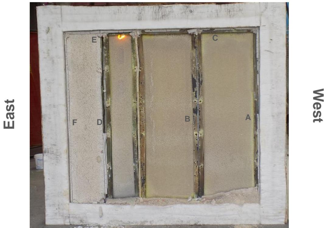
Figure 17 Exposed face of the specimen at the end of the test
