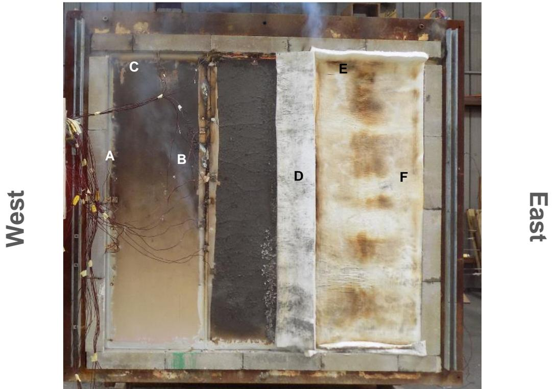
Figure 16 Unexposed face of the specimen at the end of the test
