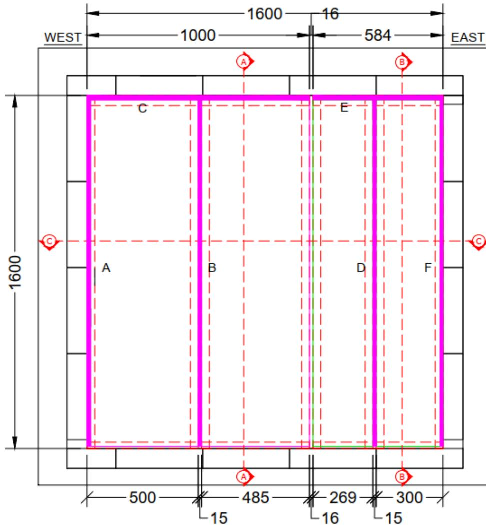
Figure 1 Elevation view of test specimen (unexposed side)
