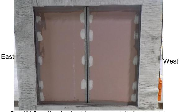
Figure A6.2: Exposed face of specimen before commencement of the fire-resistance test
