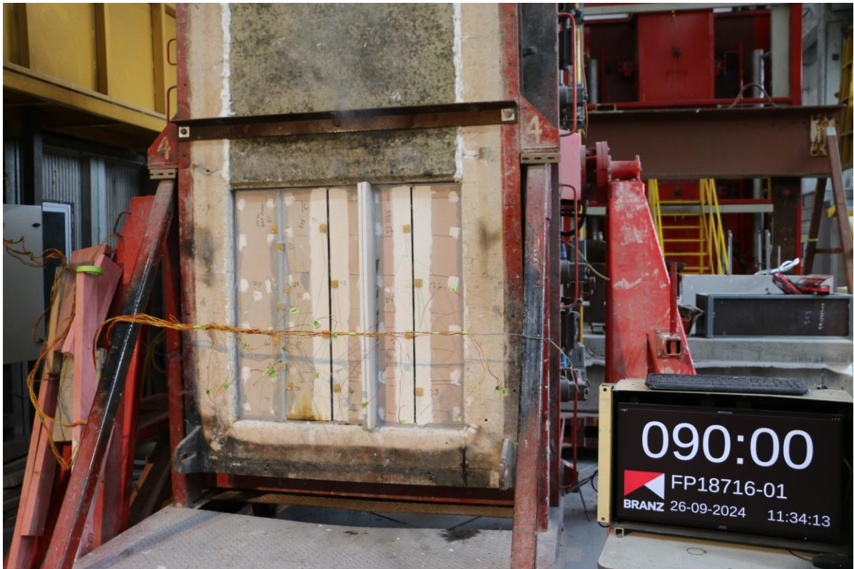
Photo 6: The Unexposed Face of the Test Assembly After a Duration of 120 Minutes
