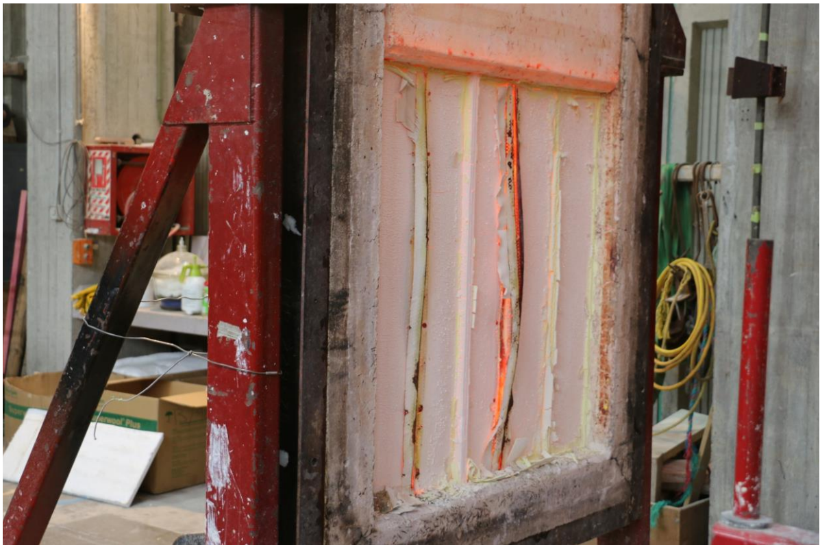
Photo 8: The Exposed Face of the Test Assembly Immediately After Testing
