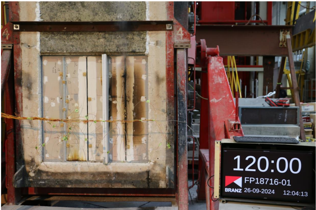
Photo 6: The Unexposed Face of the Test Assembly After a Duration of 120 Minutes
