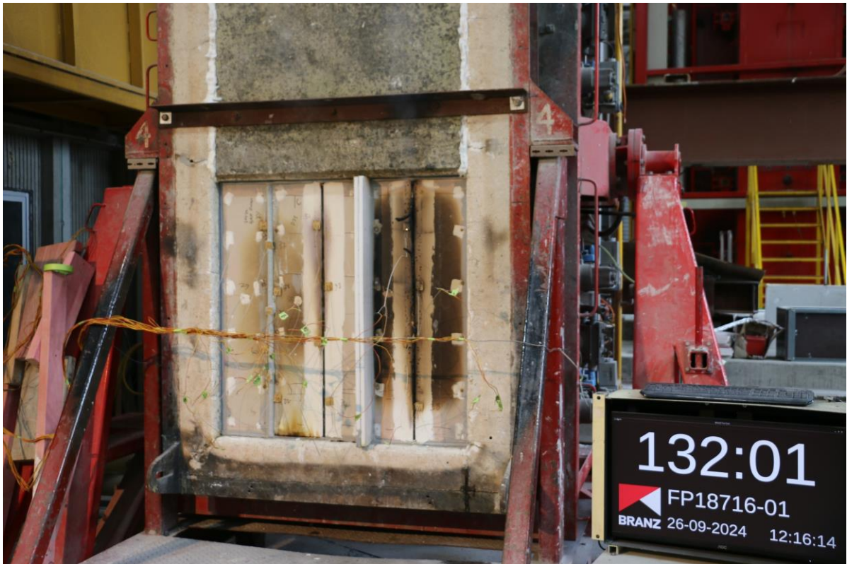
Photo 8: The Exposed Face of the Test Assembly Immediately After Testing
