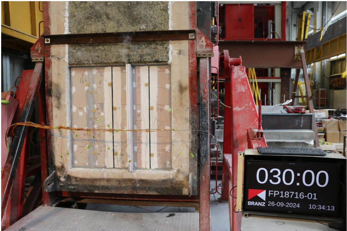
Photo 4: The Unexposed Face of the Test Assembly After a Duration of 60 Minutes
