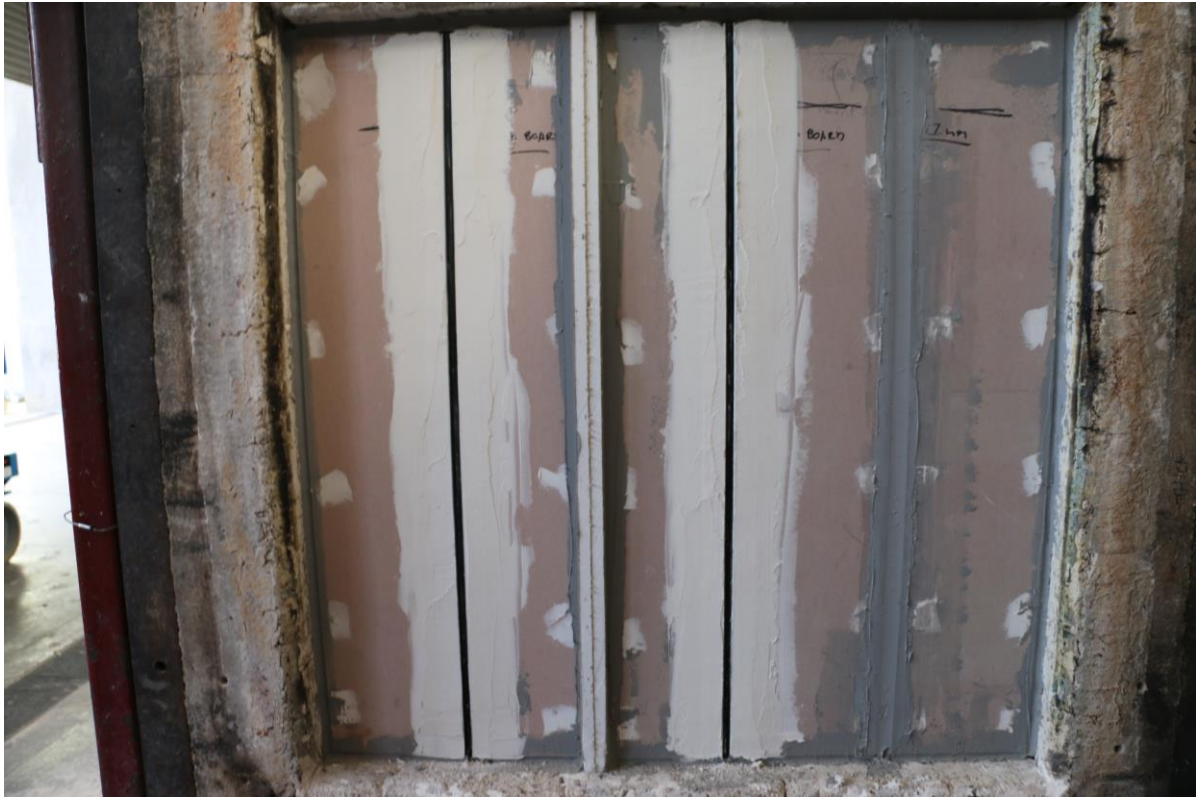
Photo 2: The Unexposed Face of the Assembly Prior to Testing
