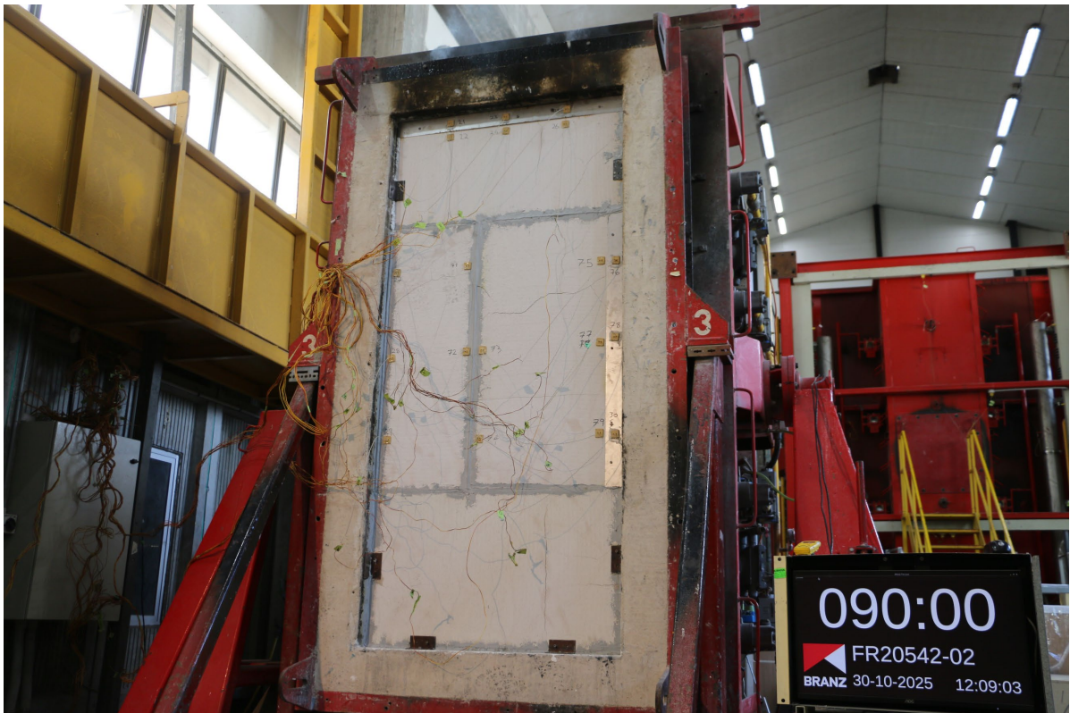
Photo 4: The Unexposed Face of the Test Assembly After a Duration of 90 Minutes
