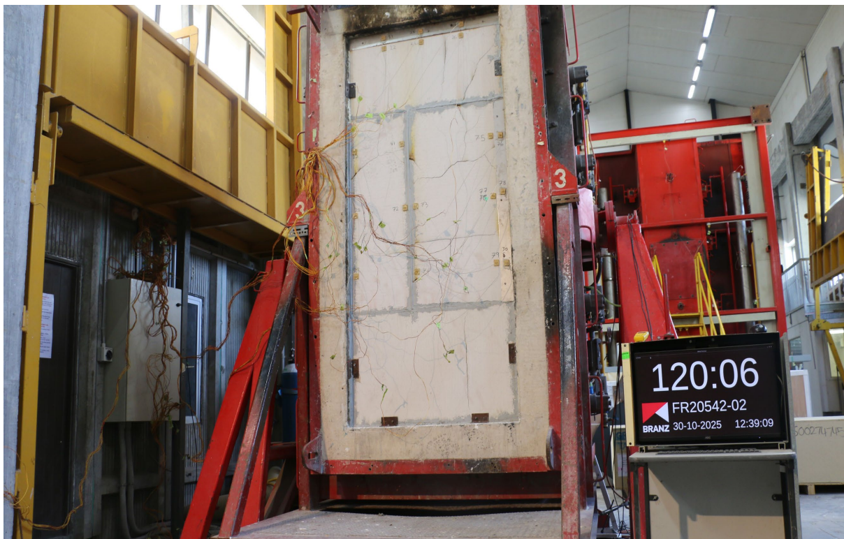
Photo 6: The Exposed Face of the Test Assembly Immediately After Testing
