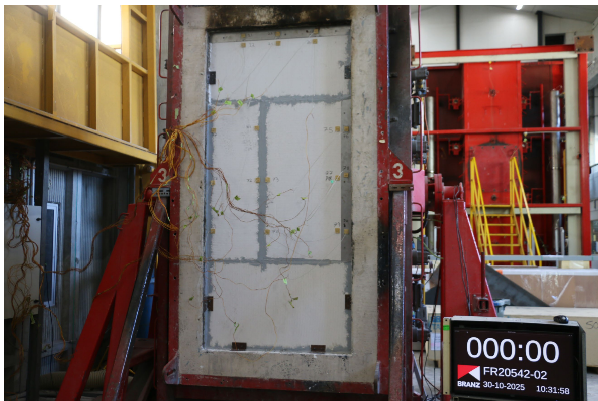
Photo 2: The Unexposed Face of the Test Assembly After a Duration of 30 Minutes
