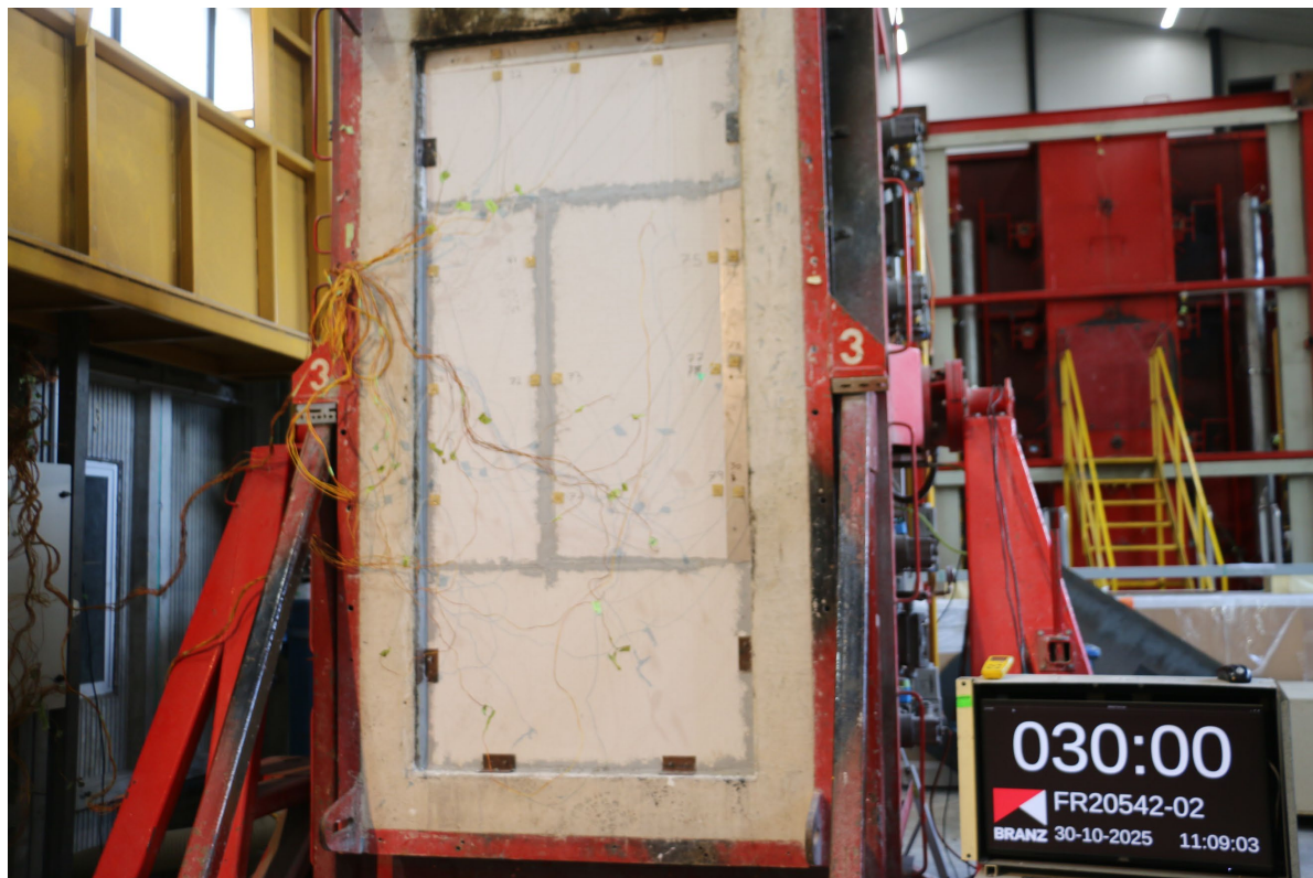
Photo 2: The Unexposed Face of the Test Assembly After a Duration of 30 Minutes
