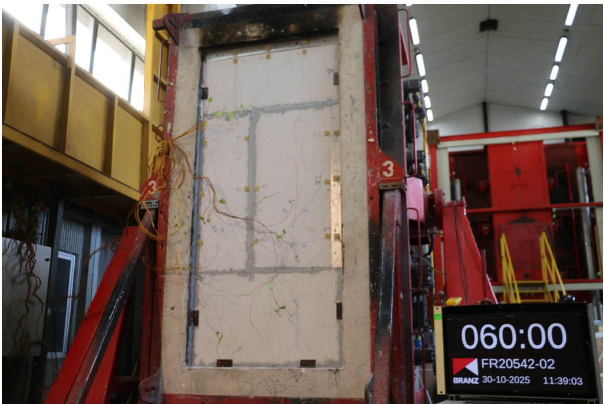
Photo 4: The Unexposed Face of the Test Assembly After a Duration of 90 Minutes
